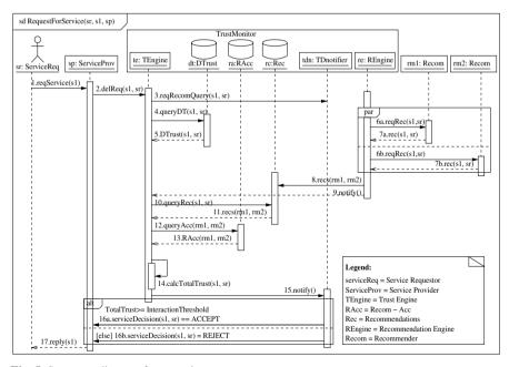
Fig. 5. Sequence diagram for a service request
